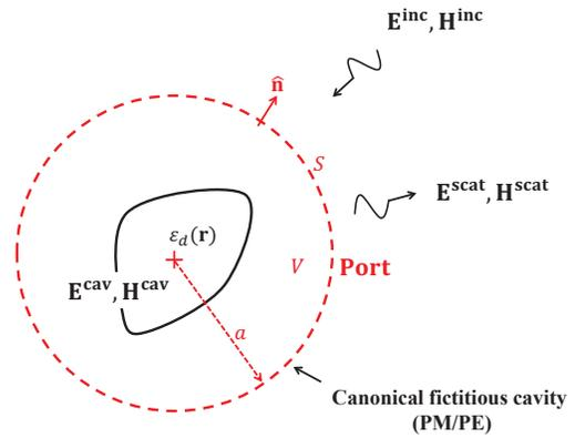
Fig. 1. General scattering problem by an arbitrary dielectric object with permittivity function  $\epsilon_d(\mathbf{r})$ , the object is enclosed by a canonical fictitious cavity with radius  $a$ , volume  $V$  and outer surface  $S$ .
