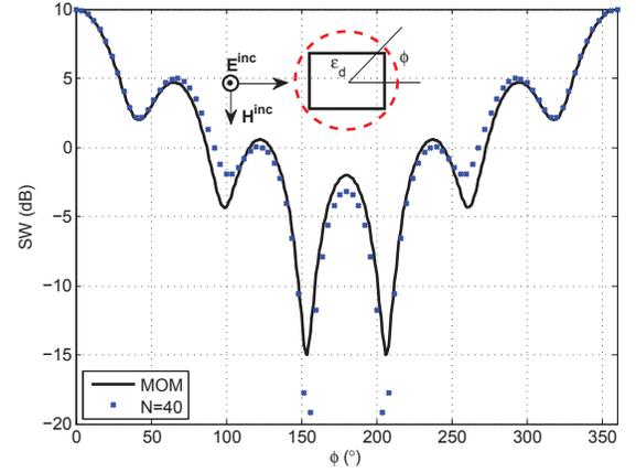
Fig. 3. SW for rectangular dielectric scatterer with  $\varepsilon_d = 4\varepsilon_0$  and dimensions  $0.8\lambda \times 0.6\lambda$  illuminated by TM<sup>z</sup> plane wave incident perpendicular to its short side with canonical cavity passing through the rectangle corners compared with the results obtained using MOM.
