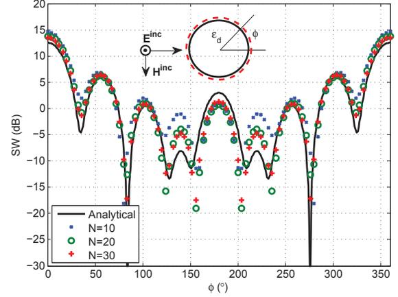
Fig. 2. SW for cylindrical dielectric scatterer with  $\varepsilon_d = 3\varepsilon_0$  and radius  $= 0.6\lambda$  illuminated by TM<sup>z</sup> plane wave with canonical cavity touching the dielectric surface compared with the analytical solution.
