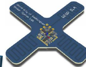
WISP: A Passively Powered RFID Tag with Sensing and Computation
