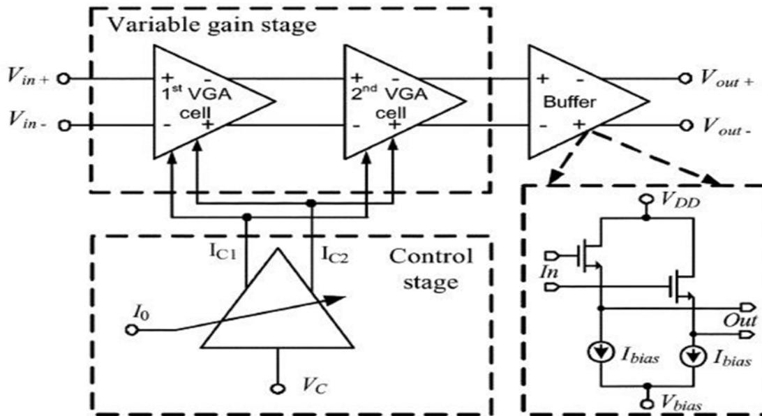
Figure 60: VGA block diagram
