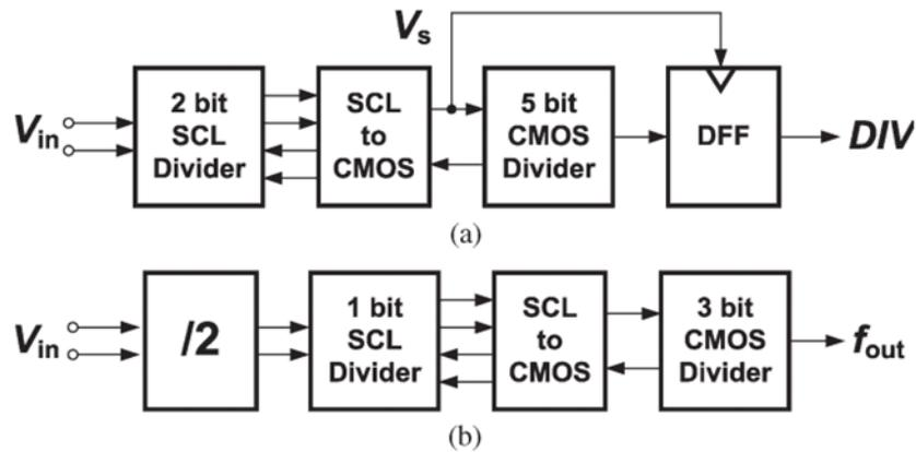
Figure 38: Multimodulus Divider Architecture
