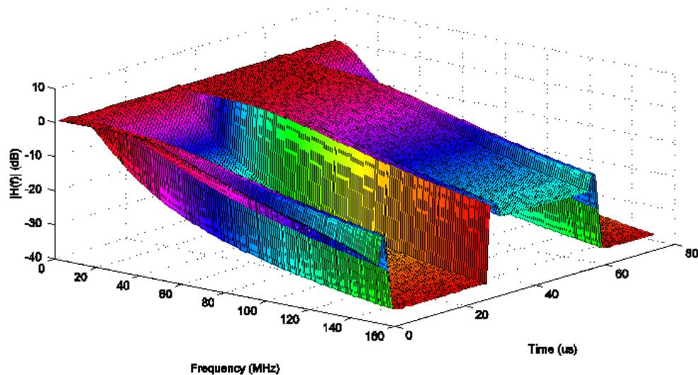
Figure 92: Prototype Filter 3D Response Curve
