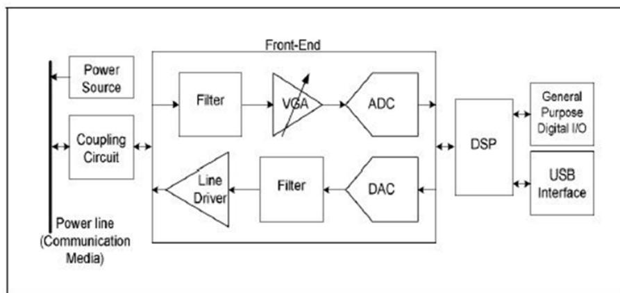
Figure 50: Typical Wireline transceiver
