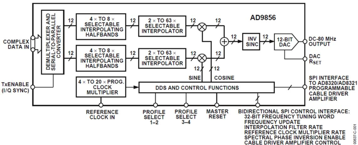
Figure 15: Functional Block Diagram of a Quadrature Digital Upconverter (Analog Devices AD9856)
