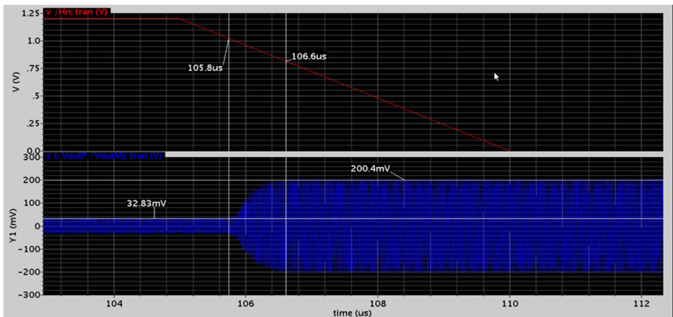
Figure 90: Filter O/P for a 30 MHz I/P Sinusoidal Signal During Hopping Transition Through Hn Control Signal
