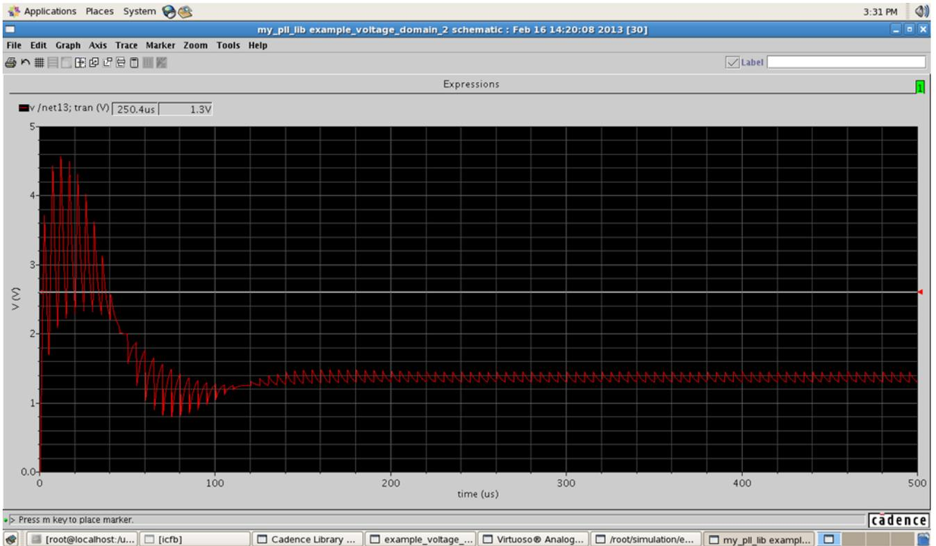
Figure 28: VCO control voltage
