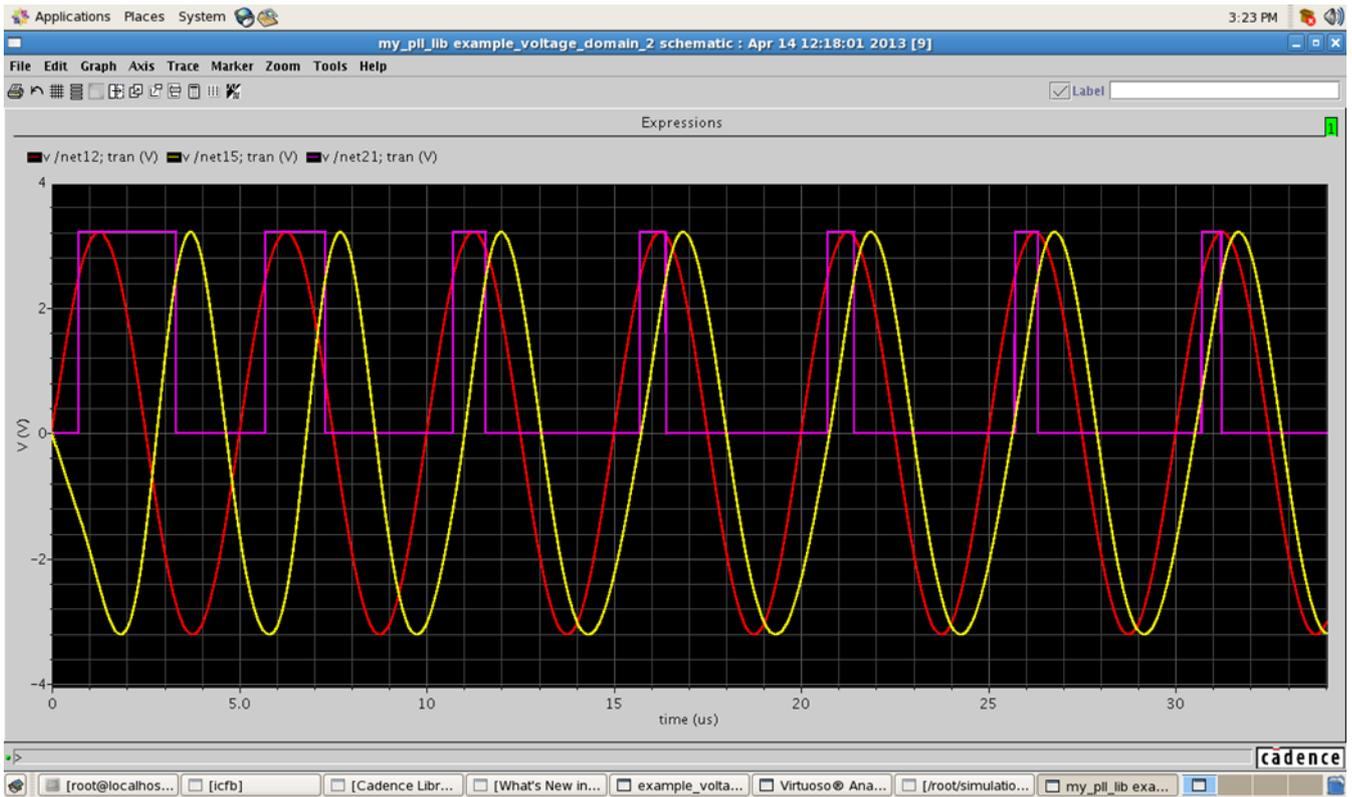
Figure 30: PFD inputs and output
