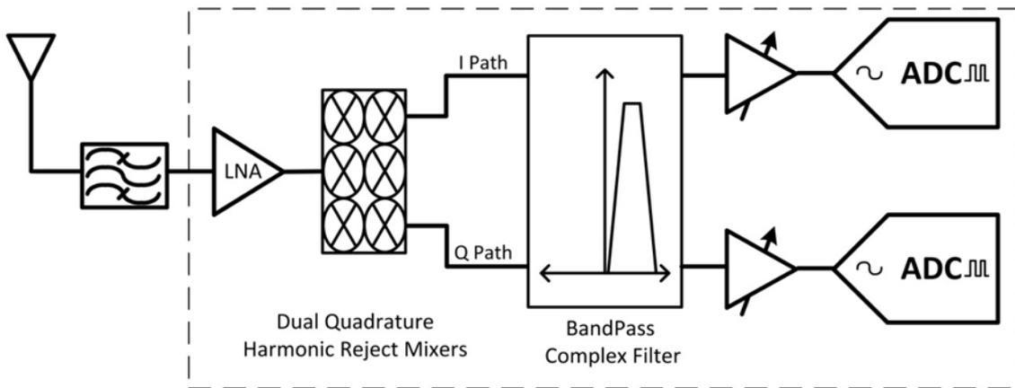
Figure 12: Proposed Receiver Block Diagram
