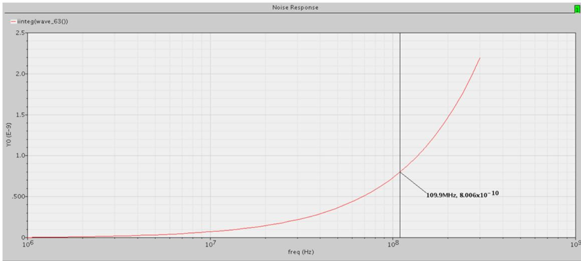
Figure 79: The total integrated input referred noise at 0 dB gain
