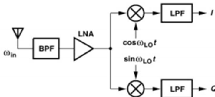
Figure 1: Direct Conversion Receiver
