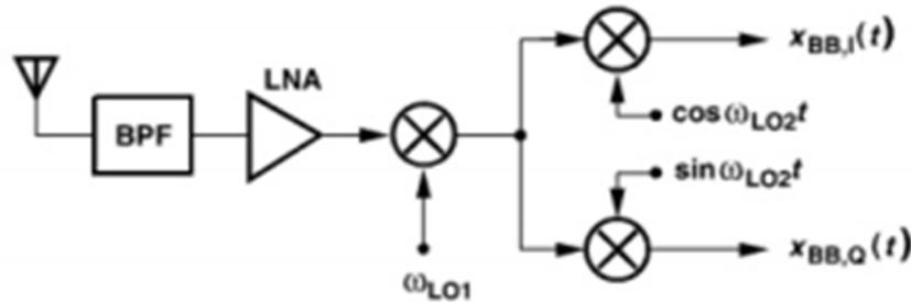
Figure 2: Heterodyne Receiver with quadrature down-conversion
