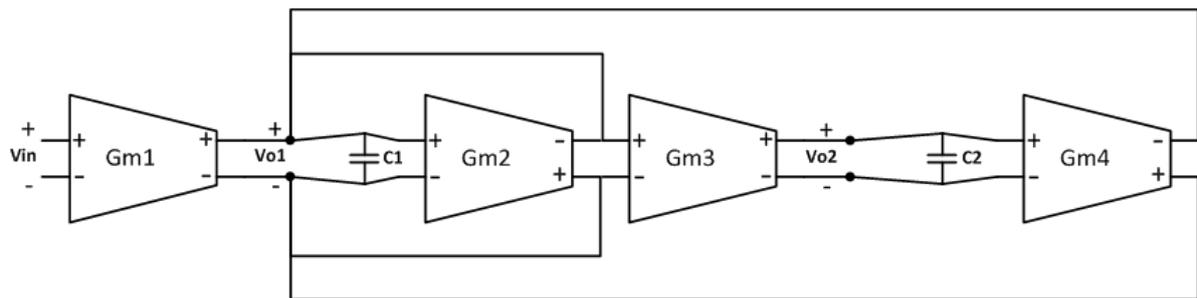
Figure 85: The Filter Preliminary Circuit Schematic
