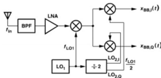
Figure 6: Divide by 2 Sliding IF Heterodyne Radio
