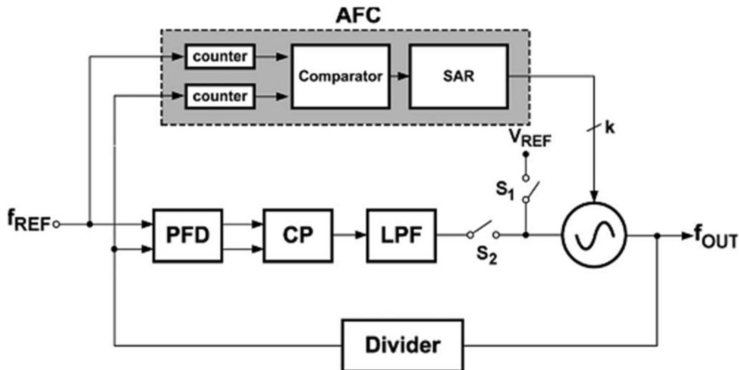
Figure 35: The block diagram of the conventional digital AFC
