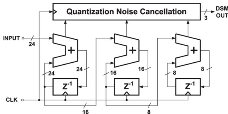
Figure 40: Block diagram of the DSM
