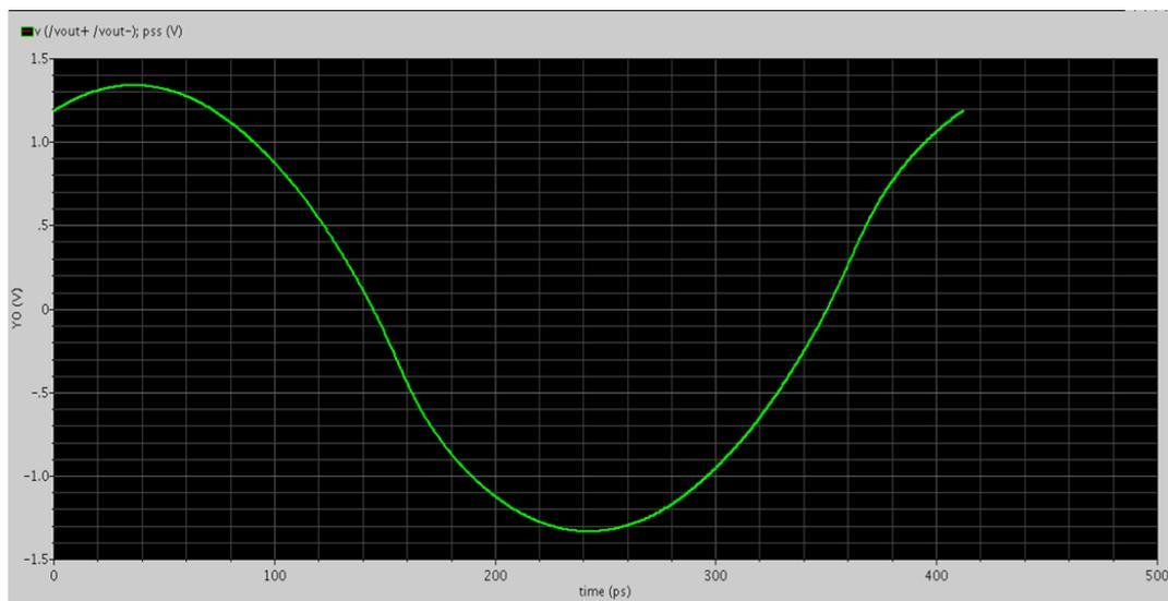
Figure 46: VCO Steady state output using PSS analysis
