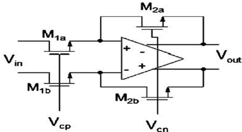
Figure 58: Inverting amp. with analog switches
