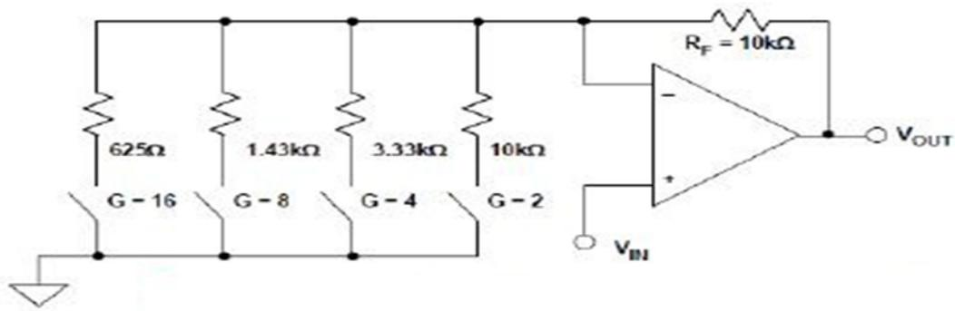
Figure 56: Non-inverting amplifier
