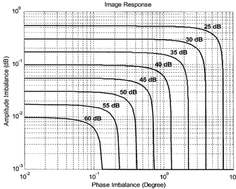
Figure 10: Image Rejection Ratio vs. Amplitude mismatch and Phase Imbalance
