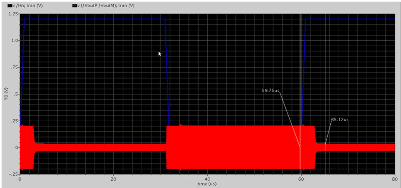
Figure 91: Filter O/P for a 30 MHz I/P Sinusoidal Signal During Hopping Transition Through Hn Control Signal
