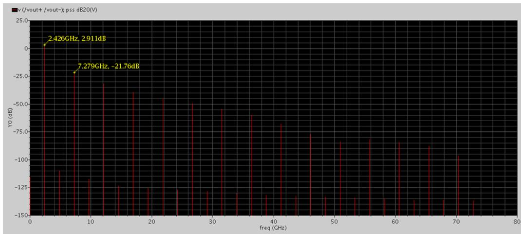
Figure 47: VCO output frequency spectrum
