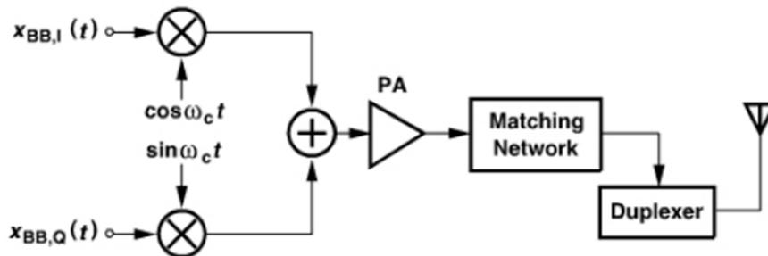
Figure 13: Direct Conversion Transmitter
