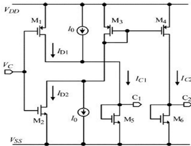
Figure 62: Schematic of the control stage
