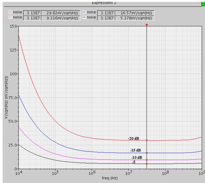
Figure 78: The input referred noise for different gain levels
