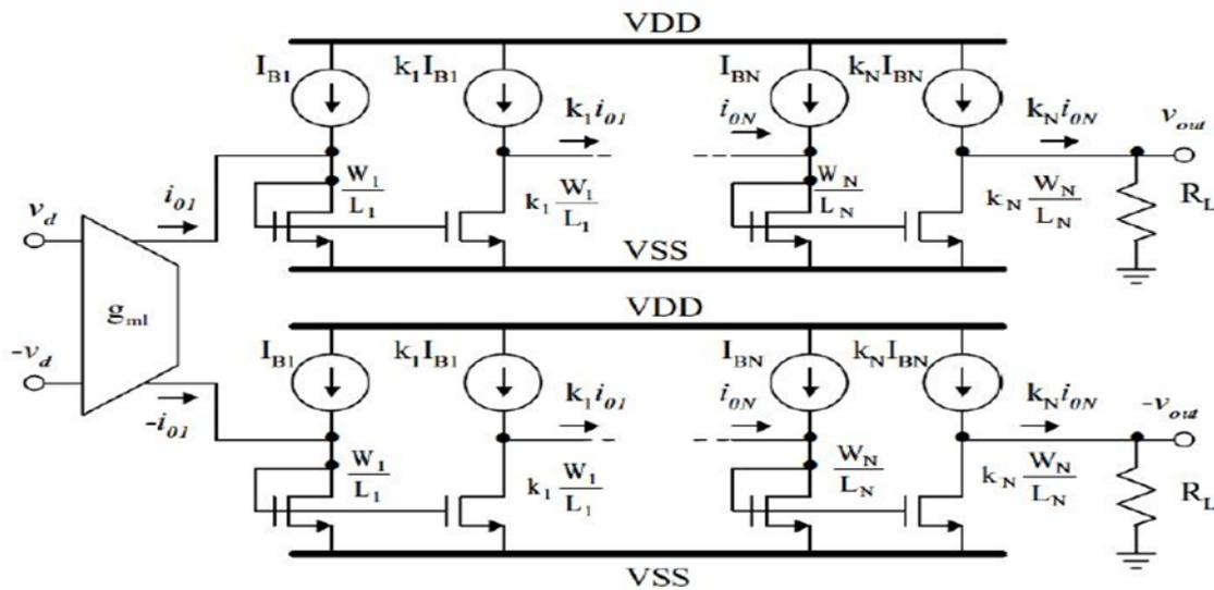
Figure 65: Analog Multiplier &amp; Current Mirror Amplifiers VGA
