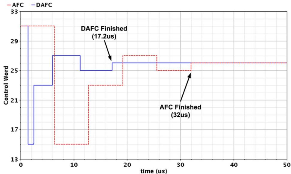
Figure 37: AFC versus DAFC simulation results
