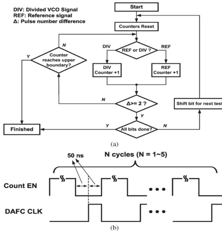
Figure 36: DAFC Flow Chart and Timing Sequence
