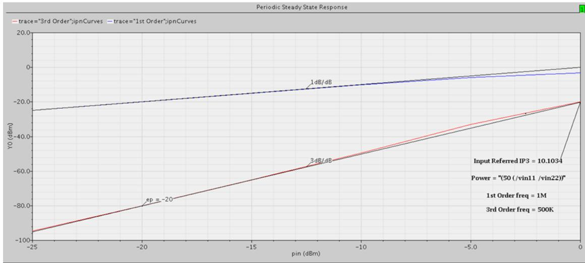
Figure 80: PSS analysis for IIP3 at 0 dB gain level
