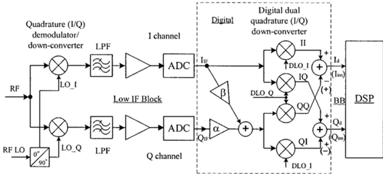
Figure 11: Digital Dual Quadrature Down-Conversion Structure
