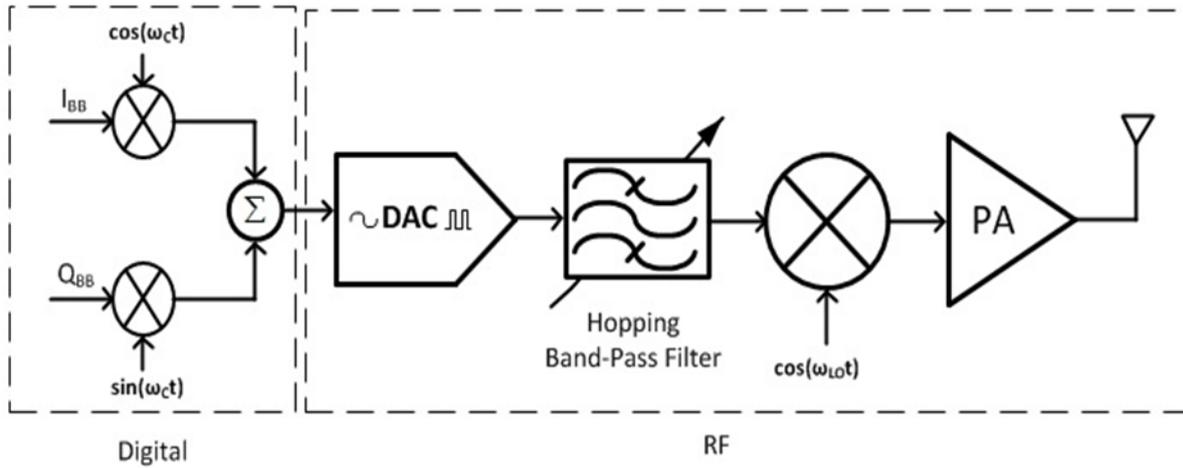
Figure 14: Proposed Transmitter Block Diagram
