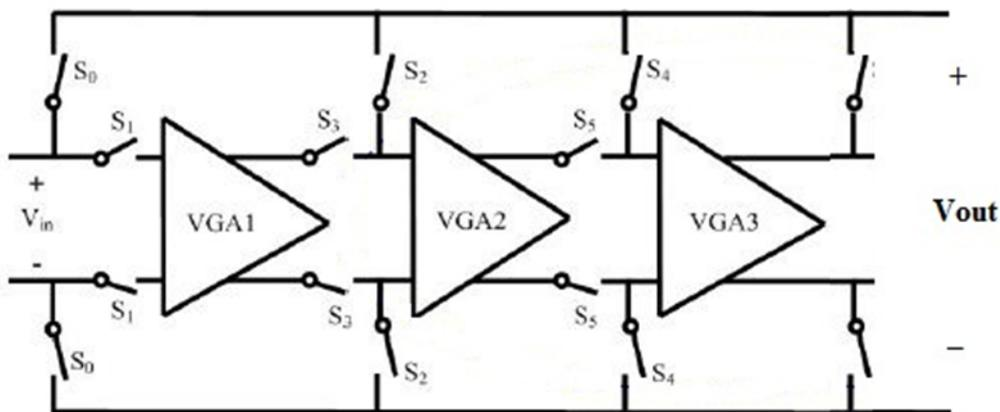
Figure 71: VGA Block diagram
