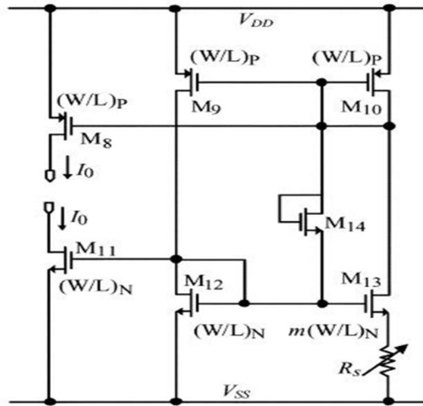
Figure 63: Circuit schematic of the current  $I_o$  generator
