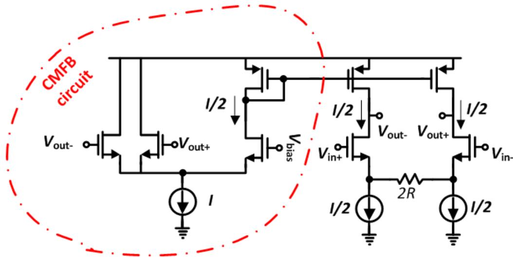
Figure 87: Used Gm Cell Architecture and the Used CMFB
