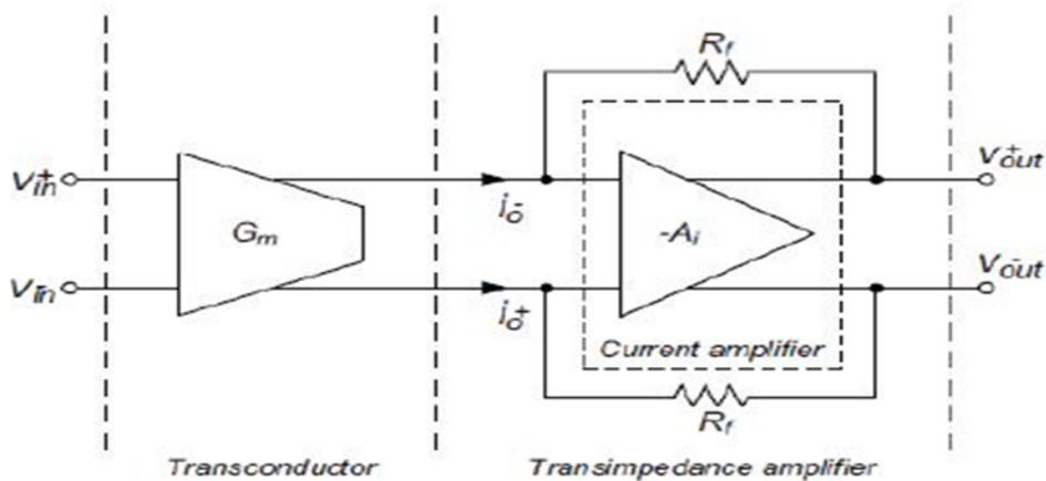
Figure 69: The Block diagram of the proposed VGA
