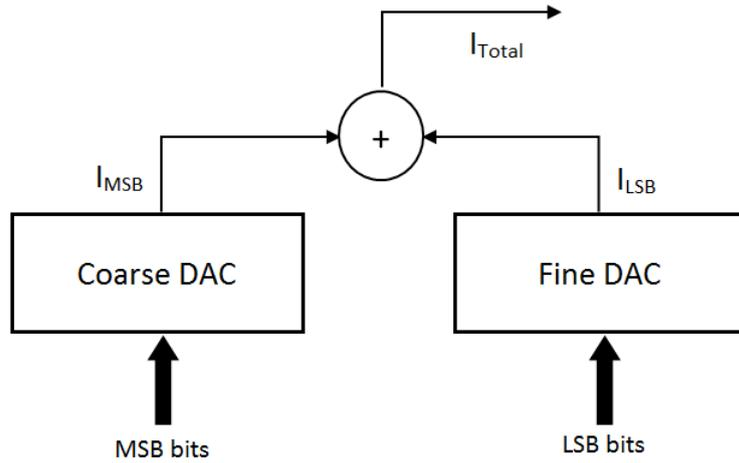
Figure 17: Architecture of segmented DACs
