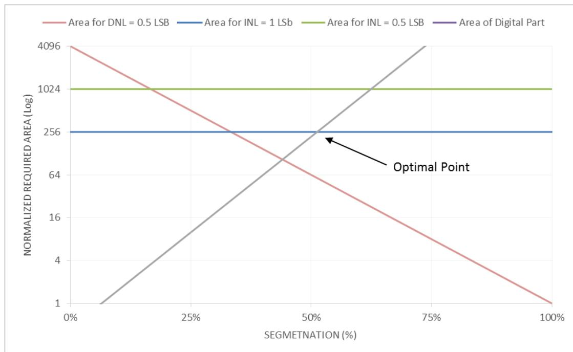
Figure 18: Normalized Required Area versus Percent Segmentation
