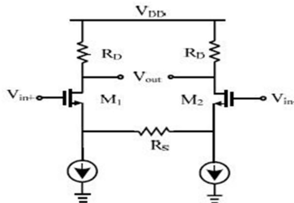
Figure 66: Differential pair with source degeneration
