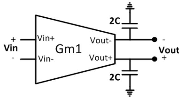
Figure 83: Basic Integrator Cell in Gm-C Architectures
