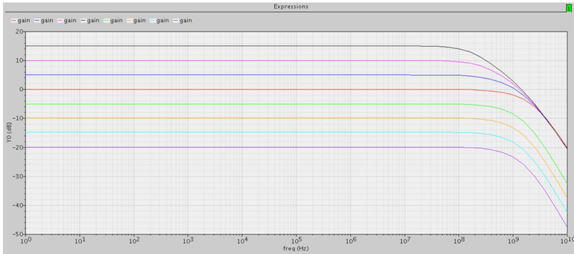
Figure 77: Frequency response of the VGA all gain levels
