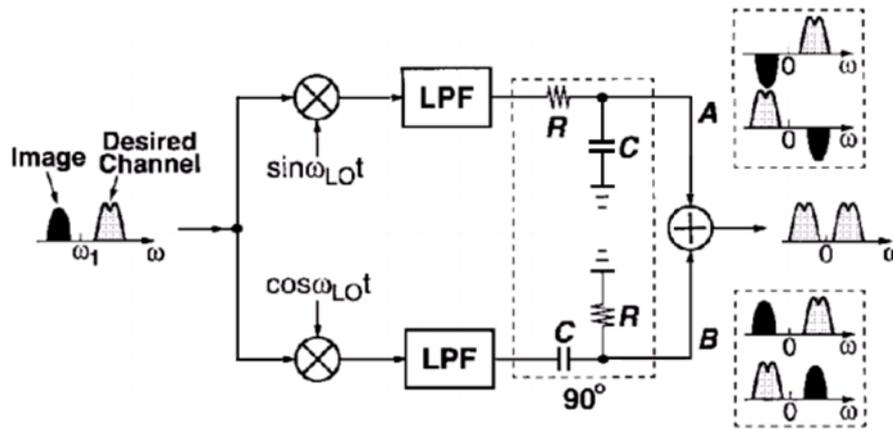
Figure 7: Hartley Image Reject Receiver
