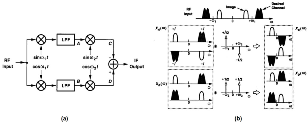
Figure 8: (a) Weaver Structure and (b) Graphical Analysis of The Weaver structure
