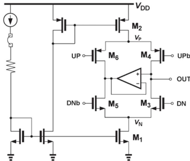
Figure 42: Charge Pump with current steering switches
