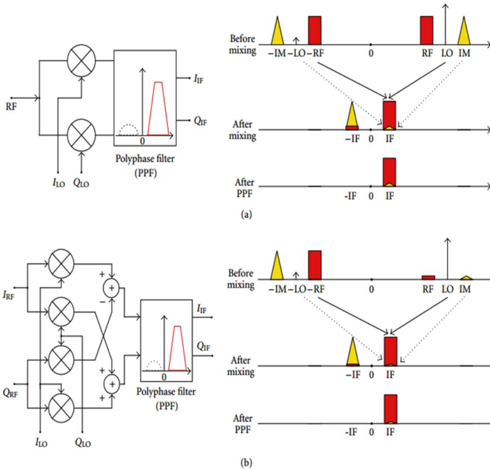
Figure 9: (a) Single Quadrature Structure and (b) Double Quadrature Structure
