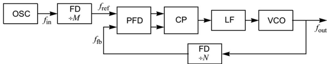
Figure 25: Typical Frequency Synthesizer Architecture
