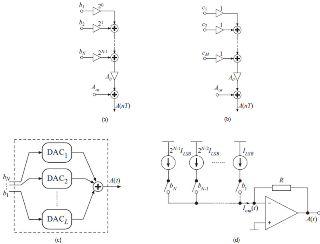
Figure 16: Different Architectures and Implementations. (a) Binary Weighted, (b) Thermometer-coded, (c) Hybrid Architecture, and (d) Current-Steering DAC
