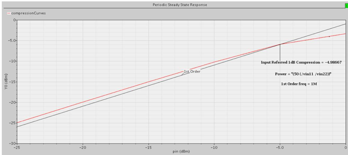
Figure 81: 1 dB compression point at 0 dB gain level
