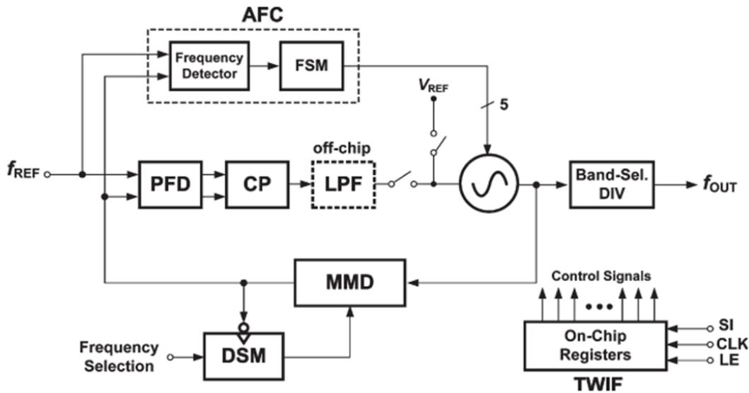
Figure 33: Implemented Frequency Synthesizer Architecture
