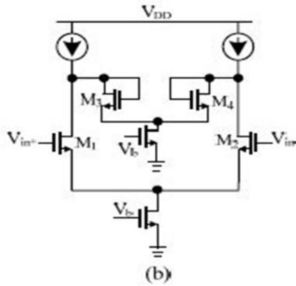
Figure 59: Differential pair with diode connected load
