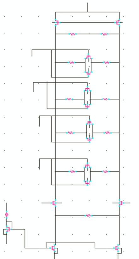
Figure 74: The main Core of VGA schematic
