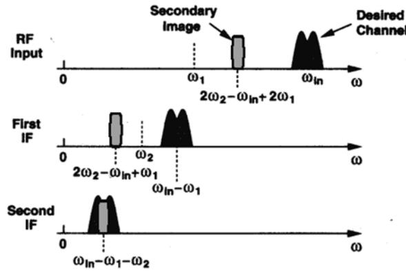
Figure 5: Secondary Image problem for Dual-IF Receivers
