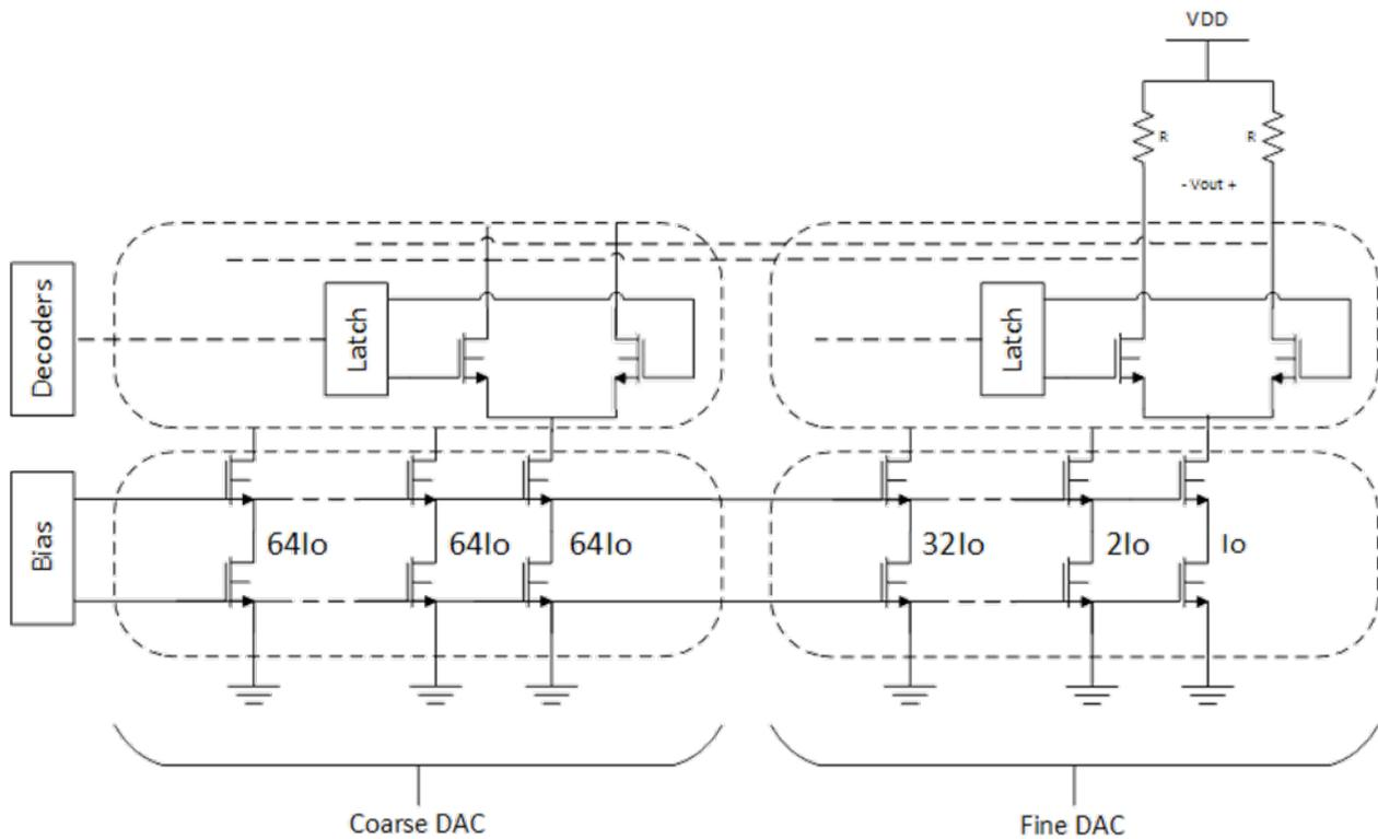
Figure 22: The Full DAC Architecture
