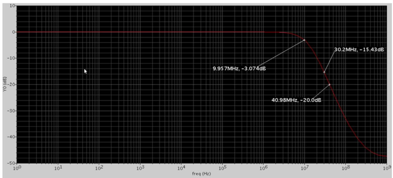
Figure 88: 10-MHz Cut-off Filter
