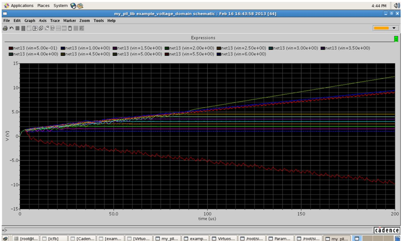
Figure 32: VCO control signal ranges
