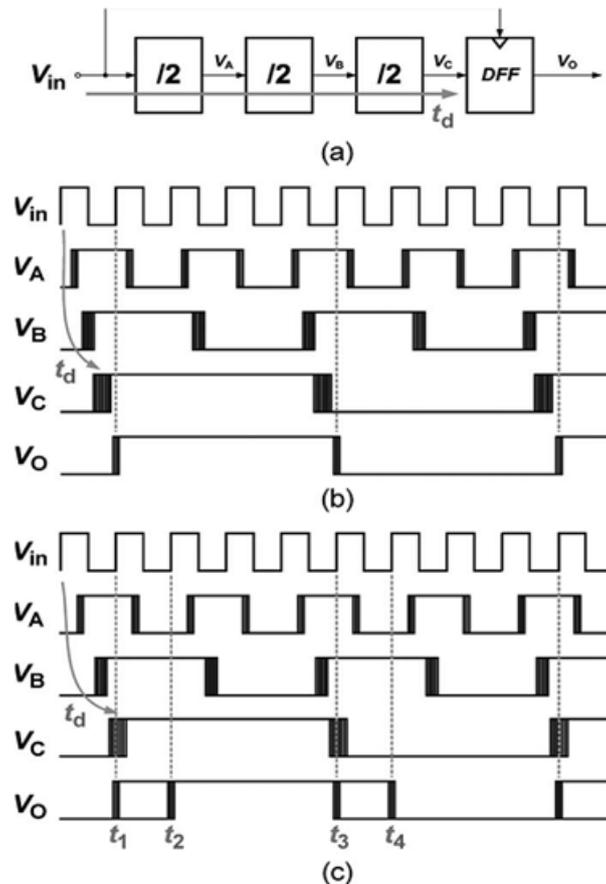
Figure 39: Metastability (a) A divide-by-eight circuit with retiming DFF. (b) Divider operation with small  $t_d$ . (c) Divider operation with large  $t_d$
