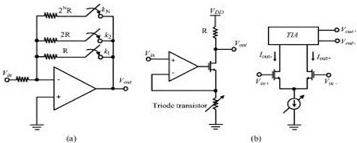
Figure 55: (a) Digitally controlled VGA (b) Analog controlled VGA
