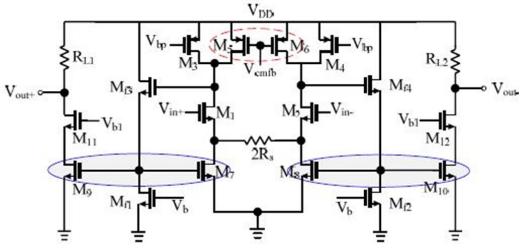
Figure 68: Full schematic of Gm boosted VGA
