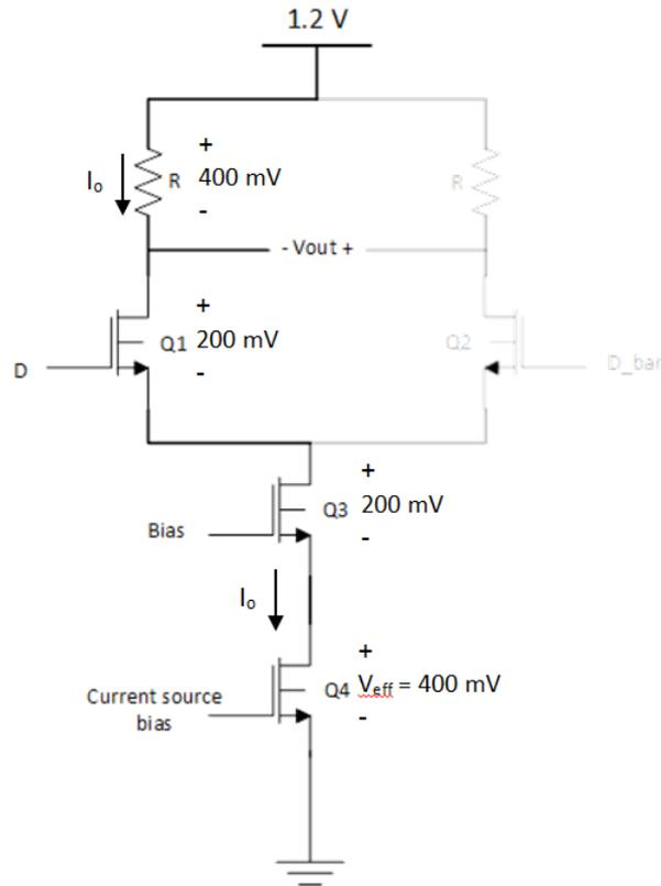
Figure 23: Unit cell with voltage distribution
