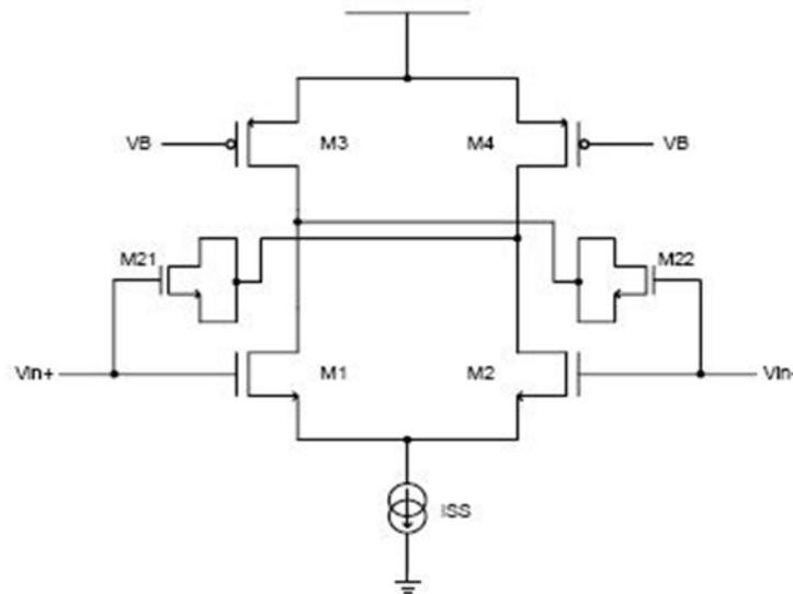
Figure 53: Capacitive neutralization with MOS transistors as capacitors
