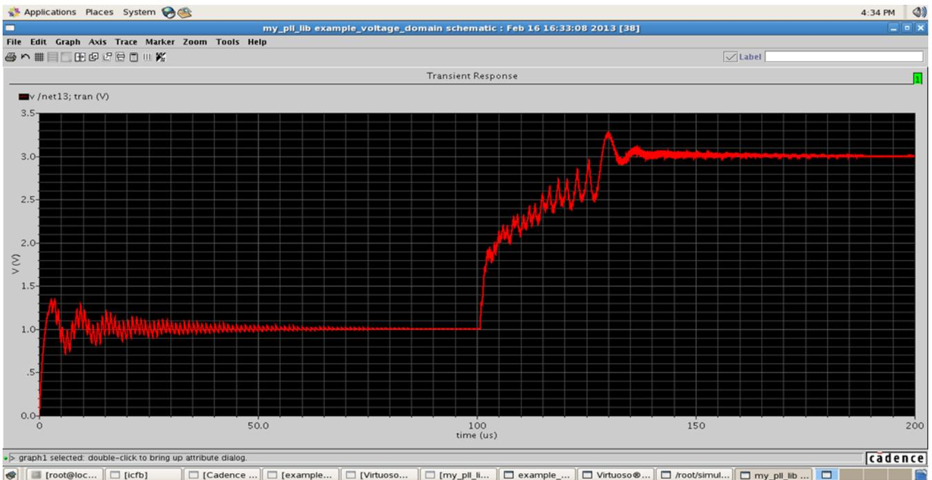
Figure 31: VCO control signal settling time
