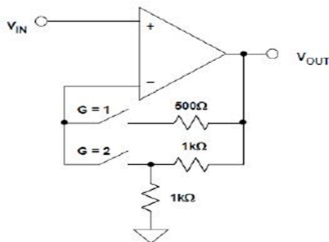
Figure 57: Alternative design of non-inverting amplifier
