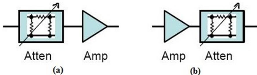
Figure 64: (a) Attenuator-Amplifier (b) Amplifier-Attenuator
