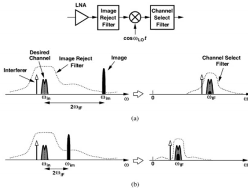
Figure 4: Trade-off between Image Rejection and Channel selection for (a) high IF and (b) low IF
