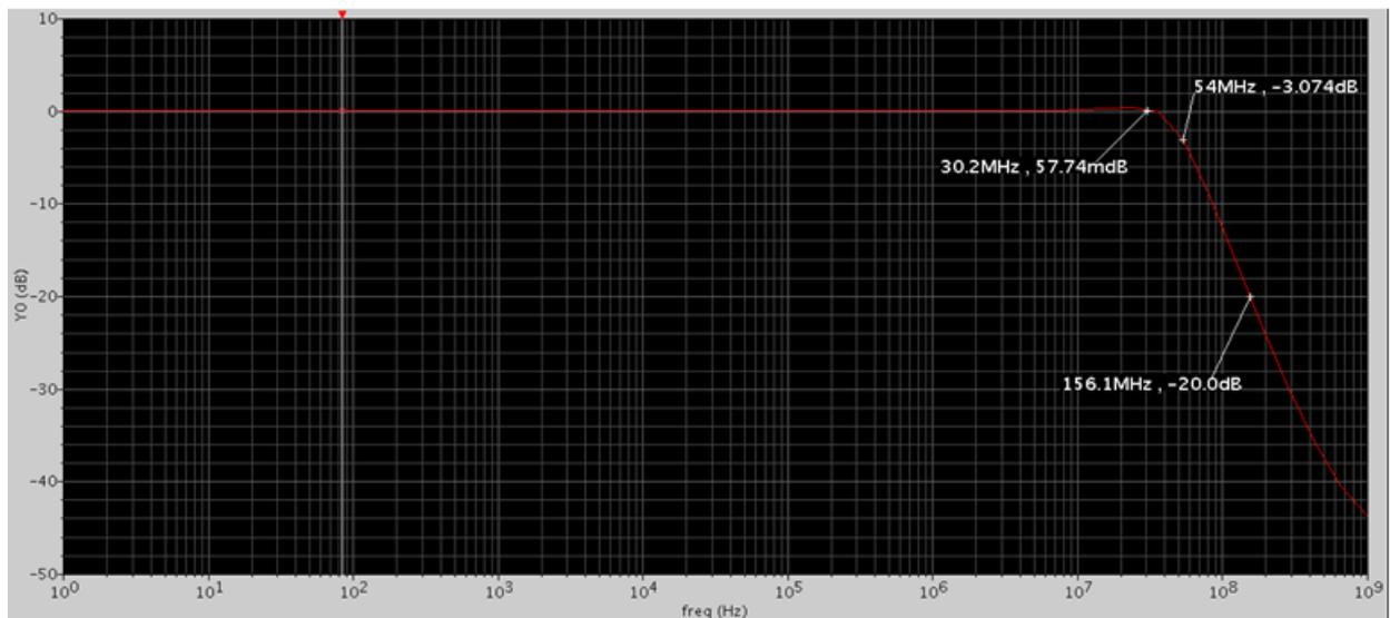
Figure 89: 50-MHz Cut-off Filter
